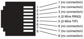
Figure 3. CopperLink Ethernet Extender (RJ-45) twisted pair line interface.
